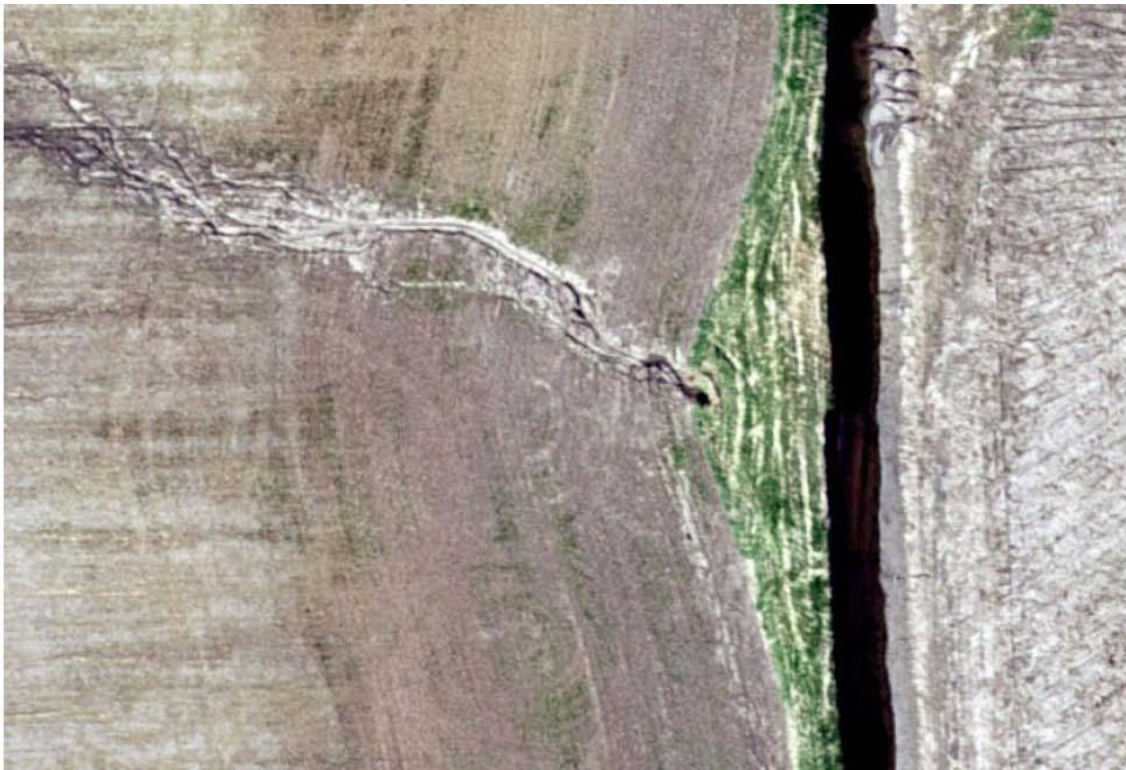
Parcel 6: A culvert at the edge of a corn/soy field in the Lake Springfield watershed has runoff leaving the field in channel flow, bypassing the buffered area and dumping directly into a nearby waterway.
