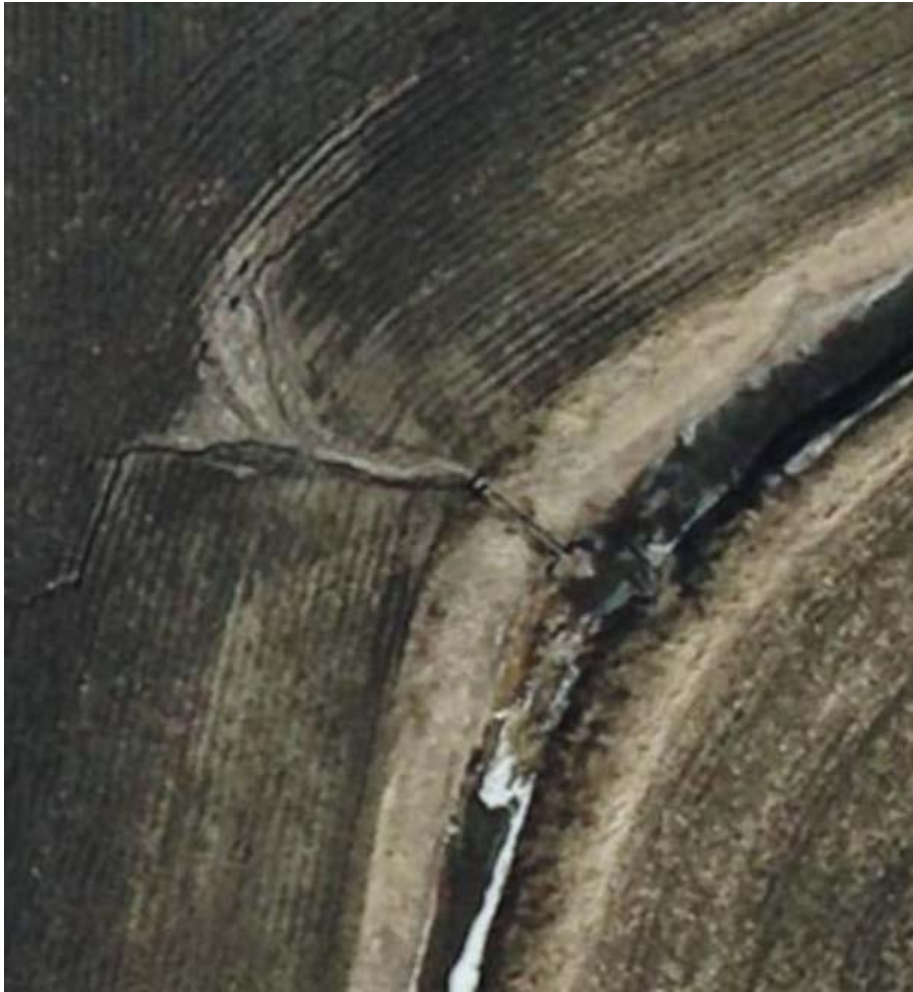
Parcel 13: A channel has formed on the edge of a cropped field in Piatt County where runoff from the field is directed into a spillway that bypasses the existing buffer strip and dumps directly into a nearby waterway.
