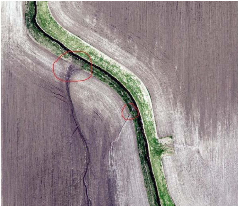
Parcel 12: High velocity runoff at the edge of a corn/soy field in the Lake Springfield watershed. This field has runoff leaving in channel flow at 2 sites (circled), appearing to run at relatively high velocity and pushing through the buffered area directly into a nearby waterway.
