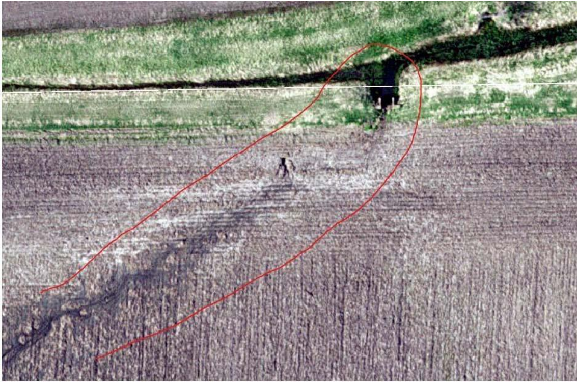
Parcel 5: Channel flow from a corn/soy field in the Lake Springfield watershed dumps directly into a nearby spillway, with the resulting erosion essentially bypassing a modest non-cropped buffer.
